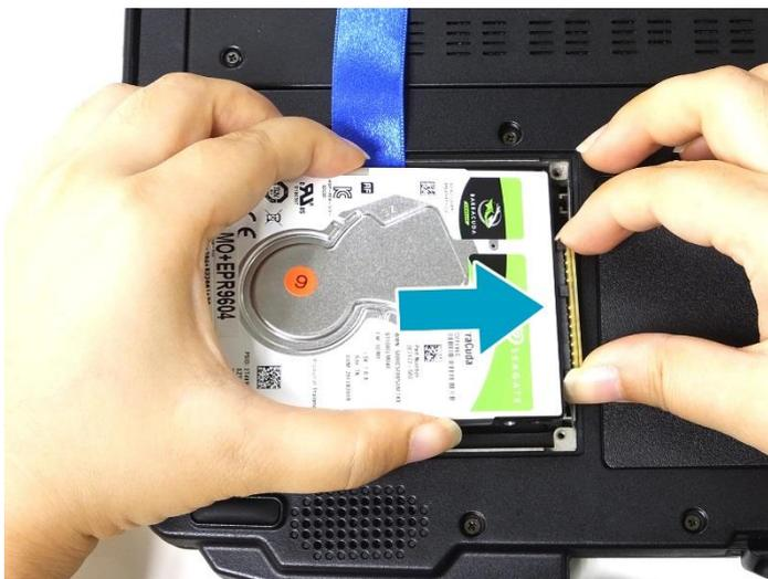
6. Lower the HDD module into its compartment.
