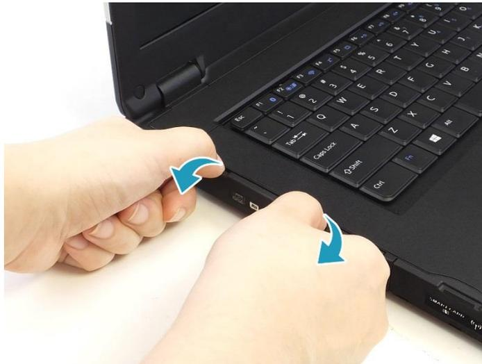
2. Press the **Eject** button to eject the tray.
