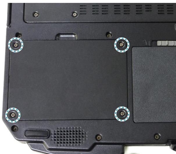
2. Remove the HDD compartment door.
