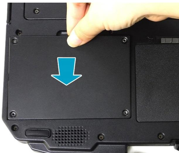
8. Secure the HDD compartment cover to the device with the screws.
