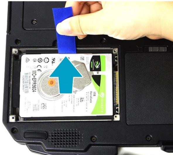
4. Disconnect the HDD module from the mainboard connector.
